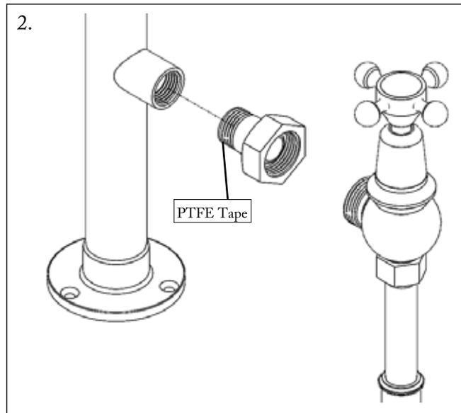
Fit the radiator valve tail thread using an appropriate allen key, use an appropriate PTFE tape on thread. **DO NOT OVERTIGHTEN.** Then loosely attach the radiator valve.
