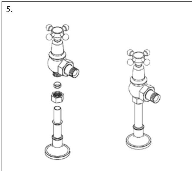
Attach the feed pipes to the radiator valves using the compression olives and nut.
