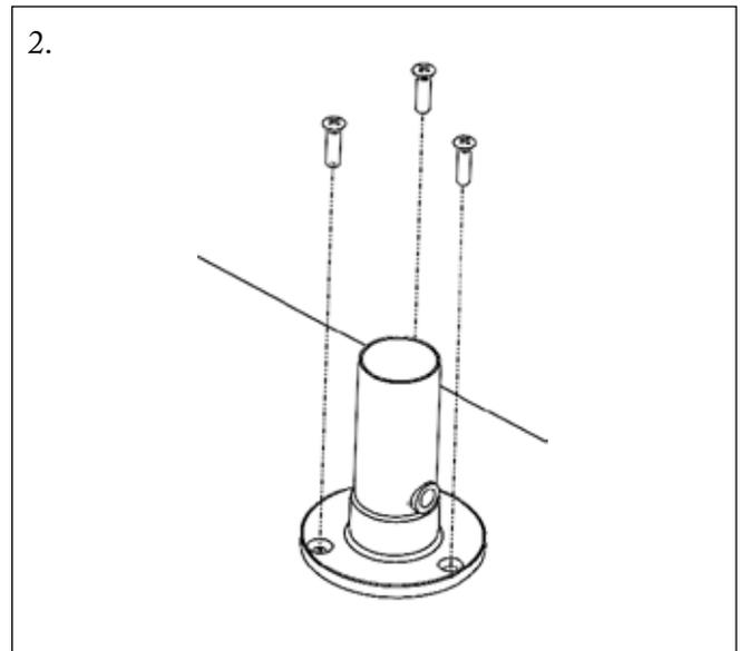
Attach false leg to the floor, ensure the false leg is in the correct location. For dual fuel models ensure that the incoming water feeds are located correctly.
