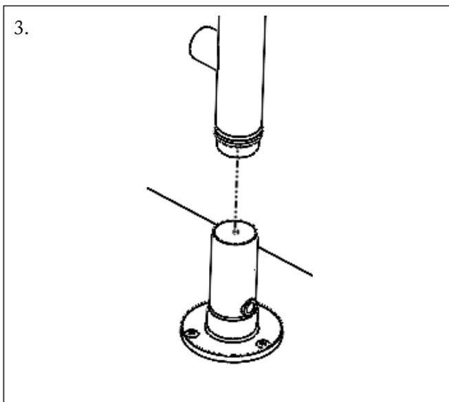
Connect the cable to the element in the towel rail. For electric models, fit the towel rail to the plugs inserted in section 1. For dual fuel models, continue to section 3.
