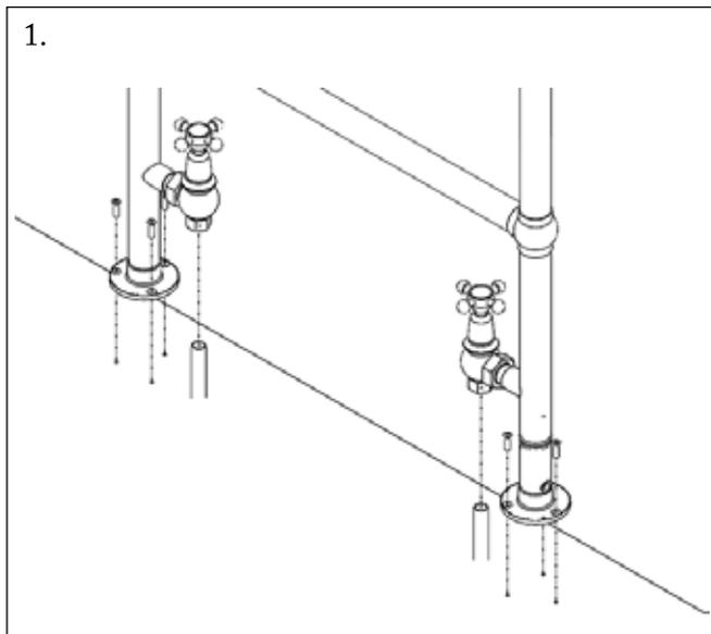
Ensure that the 15mm feed pipes are aligned correctly for fitting to the radiator valves.
