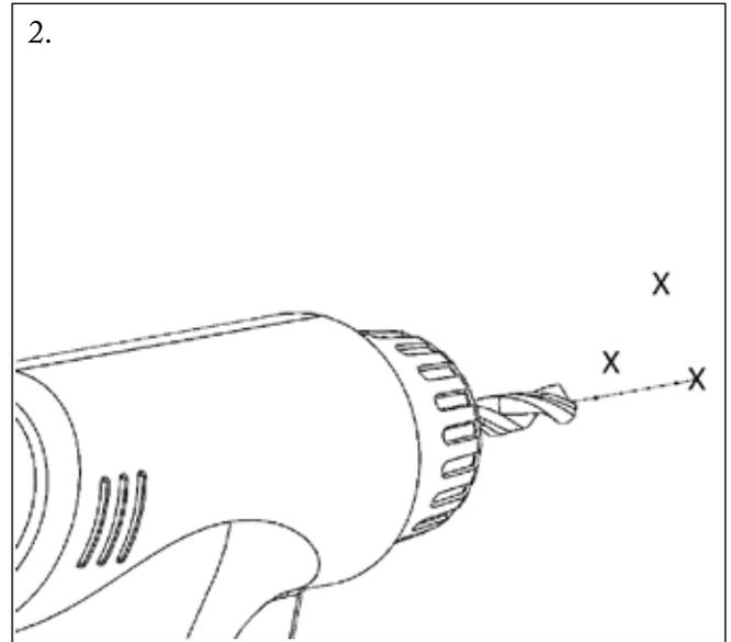
Ensure that there are no wires or pipes behind the marked locations for the fixings. Drill holes for fixings.
