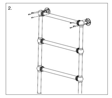
Attach the rail to the wall using the fixings inserted in section 1.
