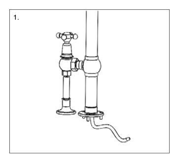
Thread electric supply cable through the hollow leg and attach to the element.
