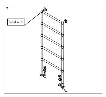
Fill the radiator and bleed using the bleed valve located under the upper left joint when looking directly at the rail.
