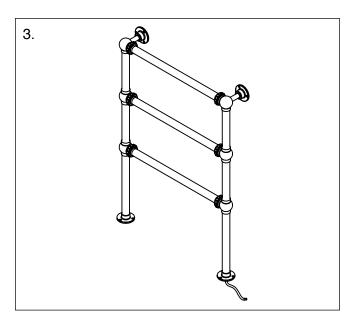
IMPORTANT: Electric elements should be fitted only by a suitably qualified electrician and must be earthed and connected to a cable outlet in the bathroom in accordance with I.E.E wiring regulations. The electrical connection should be made to a 5-amp fused fixed spur located outside the bathroom.
