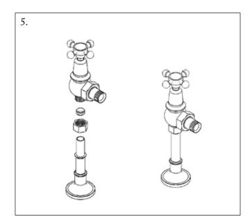
Attach the feed pipes to the radiator valves using the compression olives and nut.
