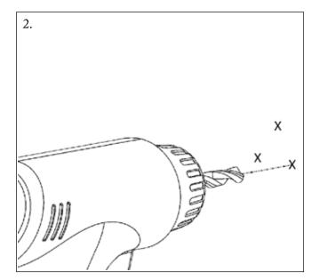
Ensure that there are no wires or pipes behind the marked locations for the fixings. Drill holes for fixings.
