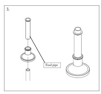
Position the escutcheon and pipe cover over the feed pipes.
